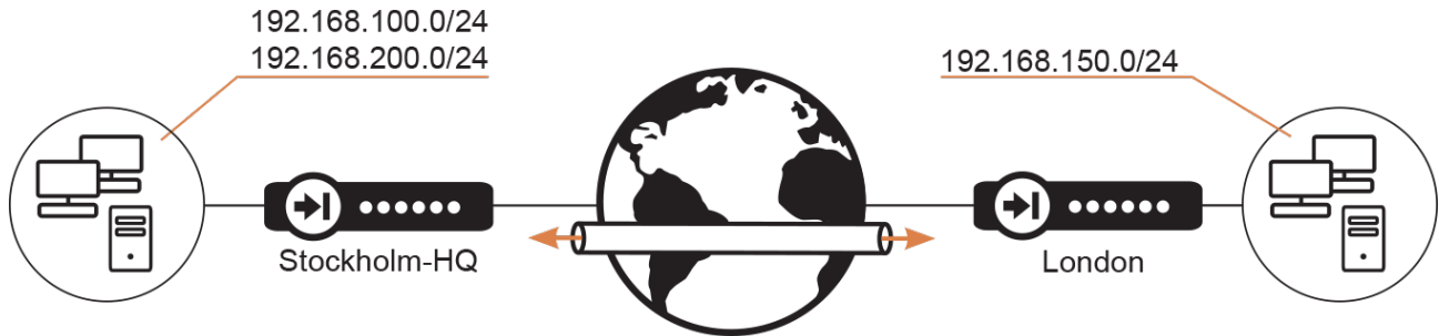
Figure 2.6.3 The tunnel network configuration from the London firewall's perspective
