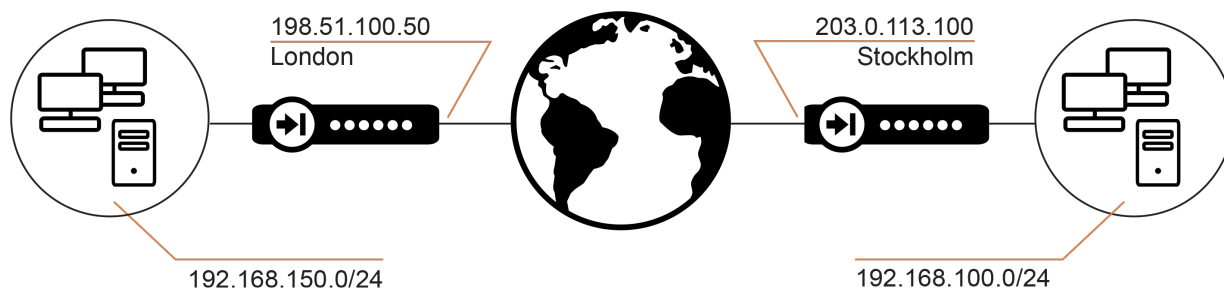
Figure 2.3.1 Adding a new IPsec tunnel interface
