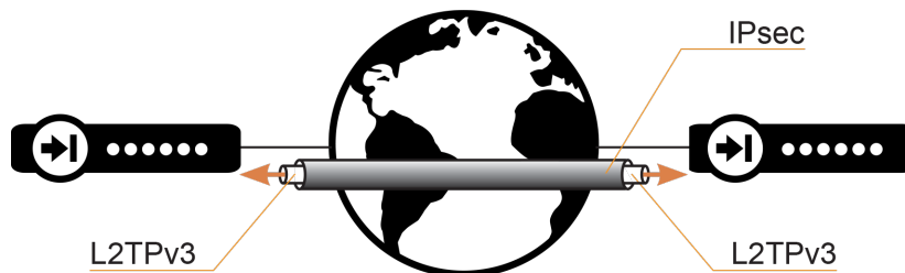
Figure 3.2.2 In order to protect the data we encapsulate the L2TPv3 traffic inside an encrypted IPsec tunnel
