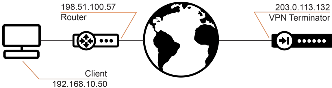
Figure 2.2.5 NAT-T needs to be used if the connecting client is behind a NAT'ing device such as a router
