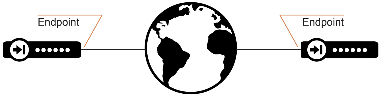
Figure 2.2.3 A tunnel endpoint means the point a tunnel is connected to. This is true for both sides, although varies slightly in case of a client/server solution
